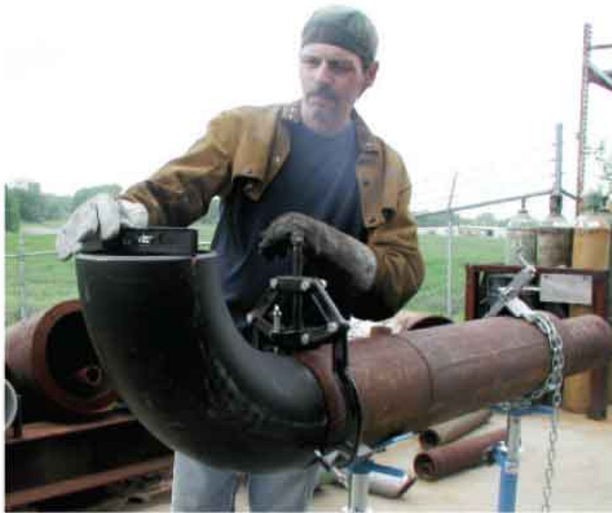
The EZ-Fit Clamp can accurately align pipe to pipe and pipe to elbow or pipe to tee as well as aligning to different diameters of pipe.
