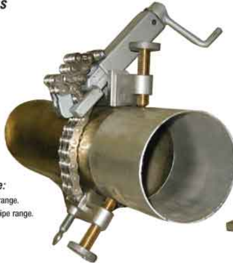
Aligns pipes to Schedule 40 Reforms pipes to Schedule 10
