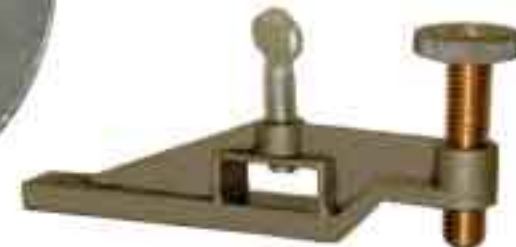
Mini-Fit Single Screw Jackbar The end of the Jackscrew is round to reduce the risk of marring the pipe.
