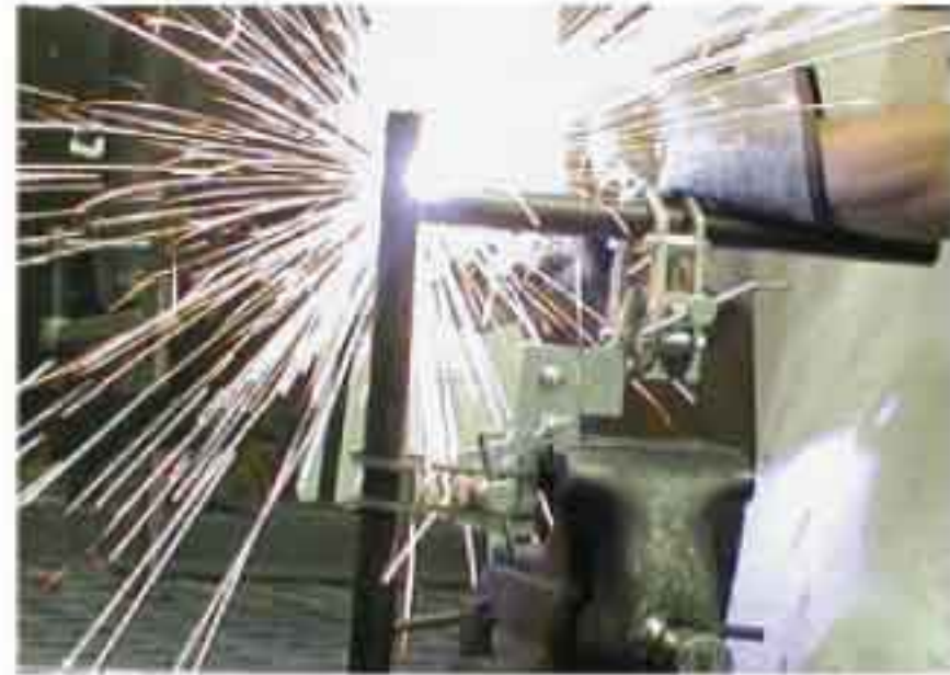
The Accu-Fit Angler allows pipes to be aligned and held in position for welding at any angle up to 90 Degrees included.
