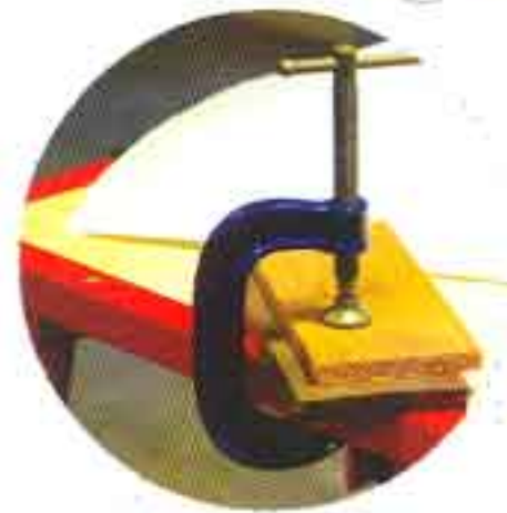
Sliding-pin handle and ball joint swivel pad.
